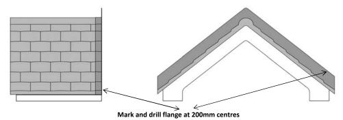
Mark out and pre-drill holes at approx 200mm centres along the canopy fixing flange (upstand).
